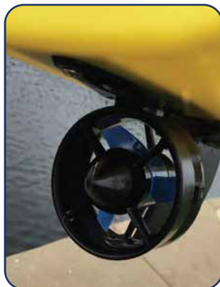
Powerful differential thrusters for maneuverability
