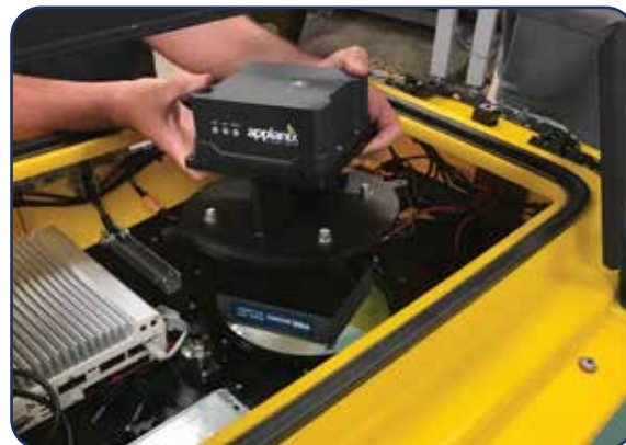
R2 Sonic Multibeam, Applanix POS MV Surfmaster and industrial PC
