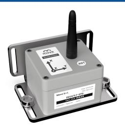
The accelerometer measures the acceleration and temperature of the exact point where it is installed in relation to the structure. It is possible to measure the vibration frequencies and carry out a modal study of the structure. All accelerometers can be perfectly synchronised with each other. Battery power supply and LoRaWAN wireless transmission. The acquisition modes can be set by the user via the web interface provided in the service.
